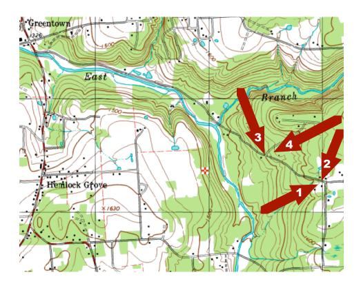
Township Road 378, Creek Road, exhibits corner sight distances at four locations that warrant 25 to 40 miles per hour speed limits to safely accommodate left and right turns, using the criteria found in Section 201.6(16)(v) of the Pennsylvania Department of Transportation regulations pertaining to Minimum Stopping Sight Distances. One of the locations identified (No. 3) is major private development roads and the others are private drives.
